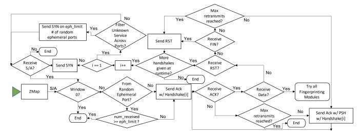
Figure 12: **LZR Algorithm**—LZR efficiently identifies real Internet services by sending application-layer data with the ACK of a TCP handshake to filter out non-acknowledging hosts and fingerprint the responding protocol.
